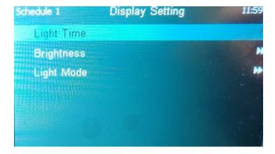
Setting light time: select the backlight time of the screen as needed, there are 6 times for option
