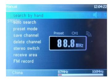
**Search by Hand**: Enter into search by hand mode, press **44** or **b** button to adjust FM channel
