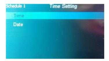
**Time:** Move the cursor to the hour/minute adjustment place, use VOL+ or VOL- button to adjust the time up or down, press Confirm button to save and exit, press ESC button to exit.
