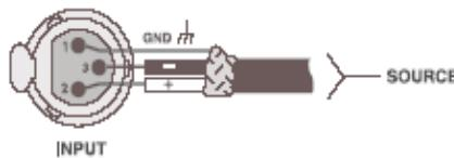
Unbalanced input connection pin diagram:
