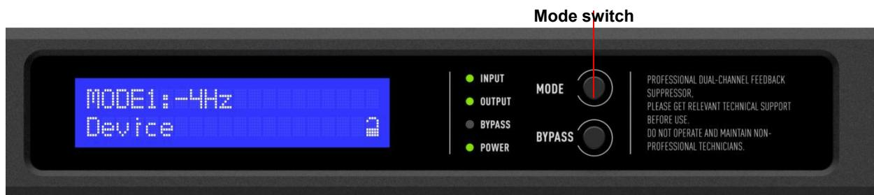
Note: The device will be silent for 3 seconds when the mode is switched!
